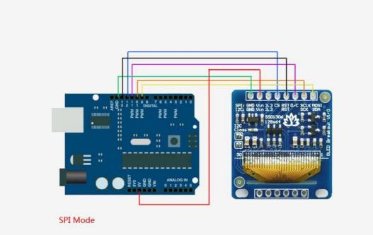
(Note: If using the display with other SPI devices, D/C, SCLK and MOSI may be shared, but CS must be unique for each device.)
